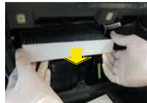
4).REMOVE CABIN AIR FILTER FROM CABIN FILTER HOUSING . REMOVE ANY DEBRIS THAT MIGHT BE PRESENT INSIDE THE CABIN FILTER HOUSING ( FIG ....)
