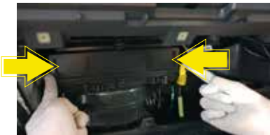
3).LOCATE CABIN AIR FILTER HOUSING BEHIND GLOVE BOX COMPARTMENT AND UNFASTEN CLIP IN THE COVER. (FIG.....)
