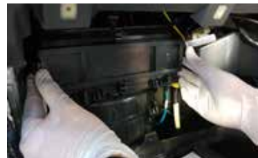
6).REINSTALL CABIN FILTER COVER ONTO HOUSING ,ENSURE COVER IS LOCKED INTO PLACE.
