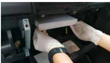
5).INSTALL CORNER FILTER CABIN AIR FILTER , MAKE SURE UP ARROW IS POINTING UP.
