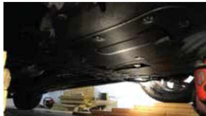
2. UNSCREW THE PROTECTOR PAD ( PLEASE CHECK THE VEHICLE MAUNAL)
