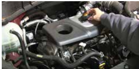
1. REMOVE THE OIL CAP , OPEN THE HOOD AND LOCATE THE OIL CAP OIN TOP OF THE ENGINE
