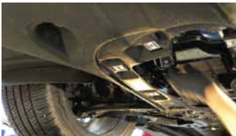
4. FIND THE ENGINE DRAIN NUT , VERIFY THAT IS THE ENGINE OIL DRAIN NUT , NOT THE TRANSMISSION DRAIN NUT
