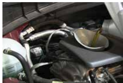
10. FILL THER NEW ENGINER OIL BE SURE TO USE THE MANUFACTURER - RECOMMEND GRADE AND VISCOSITY OF ENGINE OIL AND START THE ENGINE FOR TEST LEAK ABOUT 5 MINUTES
