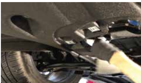
7. IT WILL TAKE SEVERAL MINUTES FOR ALL THE OIL TO DRAIN OUT OF THE CAR . PUT THE NEW GASKET FELT ON THE DRAIN NUT AND PUT THE DRAIN NUT TO ENGINE
