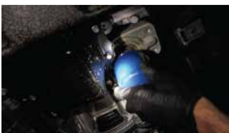
9. FILL THE ENGINE OIL TO INSIDE FILTER UNTILL FULL PLACE THE NEW OIL FILTER ONTO BASE AND TIGHTEN UNTIL THE RUBER GASKET CONNECTS WITH THE BASE , THEN GIVE IT A HALF TURN "BE CAREFUL : OVERTIGHTENING CAN SPLIT THE GASKET OR DISTORT THE FILTER"
