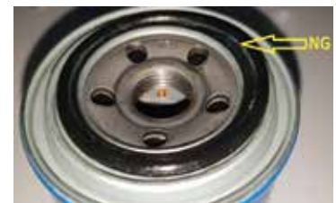
6. UNSCREW THE OIL FILTER . FIRST , TRY BY HAND THE GET A GOOD GRIP AND TWIST SLOWLY AND STEADITY , COUNTER -CLOCKWISE . IF YOU ARE UNABLE TO REMOVE THE FILTER BY HAND . YOU WILL NEED AN OIL FILTER REMOVAL TOOL TO DO THIS .
