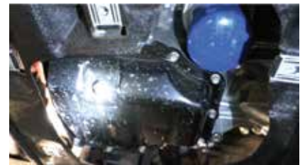
3. YOU WILL SEE OIL FILTER AND DRAIN NUT
